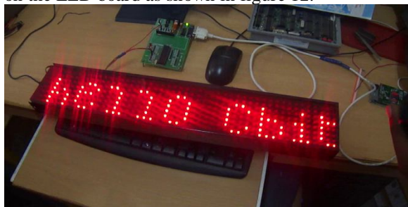
Figure 12 LED board displaying the message sent
