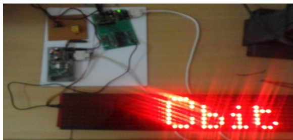
Figure 10: LED board displaying the default message
