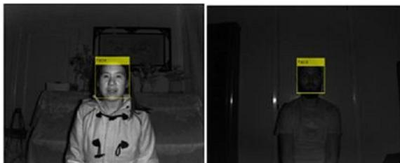
Fig. 1. True Positive Face Detection Result from various IR Images
