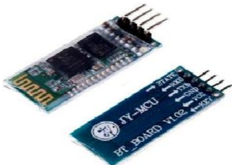
Figure 7: HC-05 Bluetooth Module
