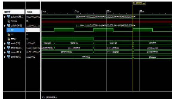
Fig 10: Error detection and correction using parity check in decoder stage
