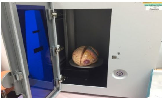
Figure 1. Instructional Object: 3D Scanning of a Human Brain Model
