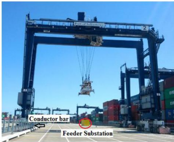
Fig.2 RTG crane in Port of Felixstowe.
