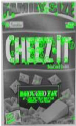
Fig. 2. Sample database image with SIFT features.
