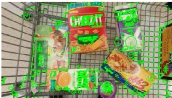
Fig. 3. Sample query image with SIFT features.
