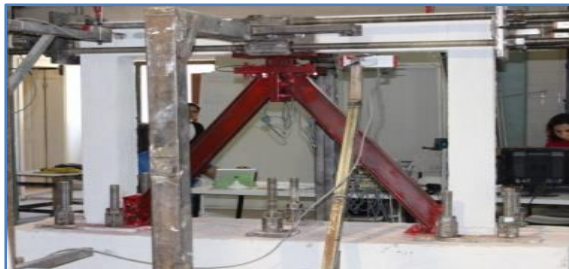
Fig.7. View of the Retrofitted sample before the test
