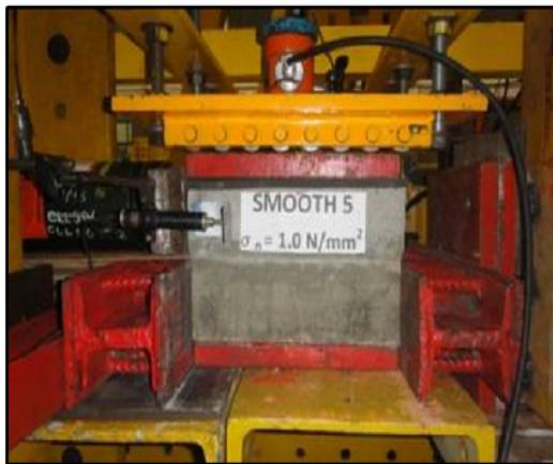
Figure 1 “Push-off” test setup
