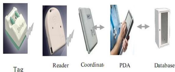
Figure 2: ZigBee Network Components
