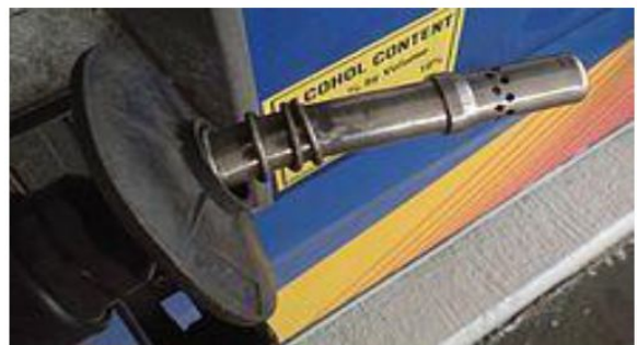
Fig.9 Gas nozzle with vapour recovery
