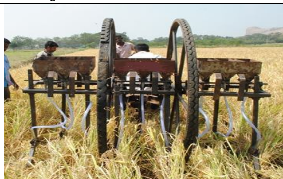
Fig.5. Rice-fallow pulse planter in operation under rice crop stand condition
