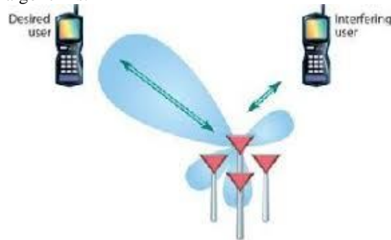
Fig shows Beam Formation in Smart Antennas
