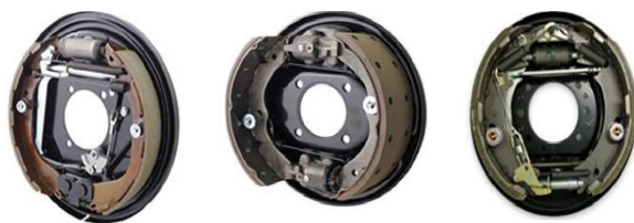
leading shoe twin leading shoe duo-servo
