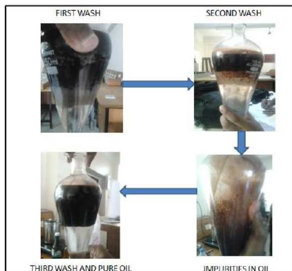
Fig 5.1 Transesterification by KOH (4g)-catalyst & ethanol-reactant
