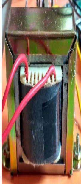
Fig4: Step down transformer
