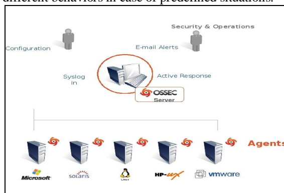
Figure 4. Basic architecture of Ossec.
