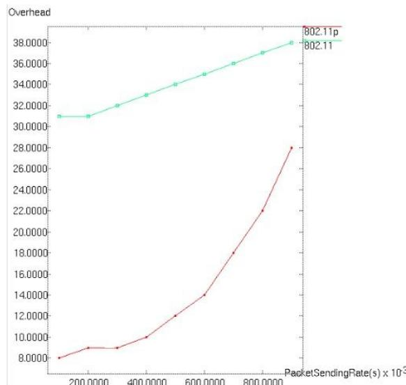
**Fig4. Routing overhead with congestion control**
