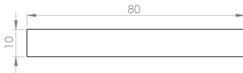
Fig.1. Specimen configuration for flexural test
