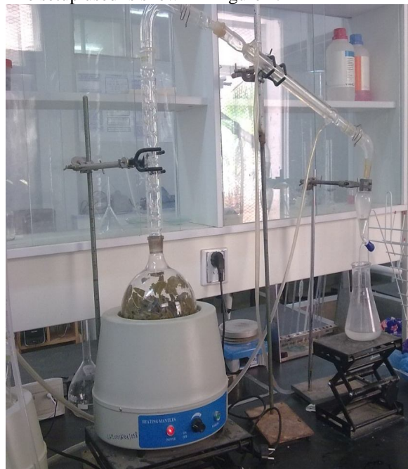
Fig.1 Installation of hydrodistillation (Clevenger apparatus) - [10]
