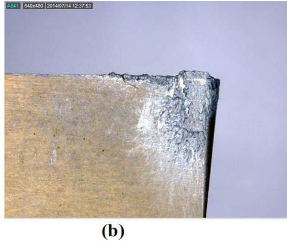
**Figure 3.** Build-up edge formation during machining (a) Bi-treated Al20%  $Mg_2Si$  composite and (b) Al20%  $Mg_2Si$  metal matrix composite.
