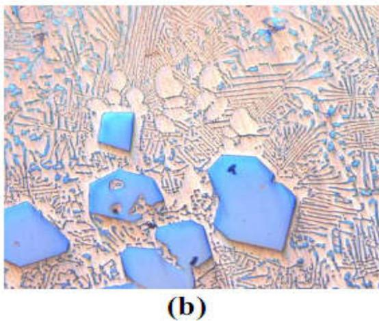
**Figure 2** Optical micrographs showing different size of  $Mg_2Si$  particles indifferent conditions (a) base composite (b) Bi-treated composite
