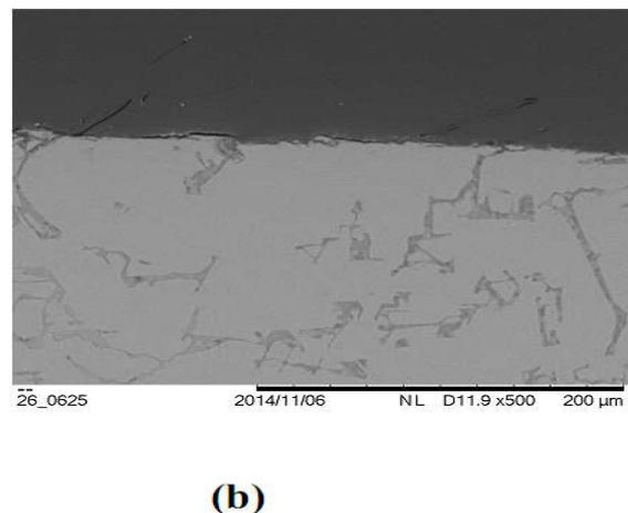
**Figure 4.** Image of machined subsurface of (a) Al20%  $Mg_2Si$  MMC and (b) Bi-treated composite.
