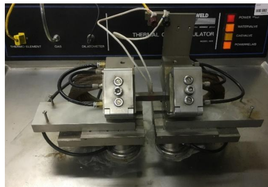
Figure 1 Thermal cycle simulator type SMITWELD used in this study, complete with sample and single thermocouple.
