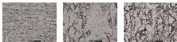
Figure 7 Carbide precipitation in duplex alloy at 700°C with time, a: 5 min, b: 30 min and c: 60 min.
