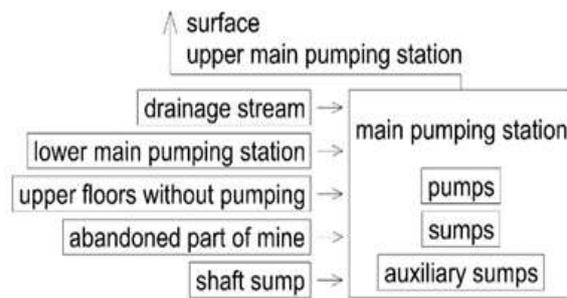
Figure 2: Block scheme of the tributaries of mine water of the main pumping station
